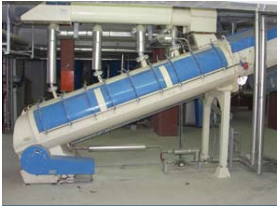
Super conditioner preparation stage on pellet mill
