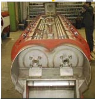
Jacket steam piping
