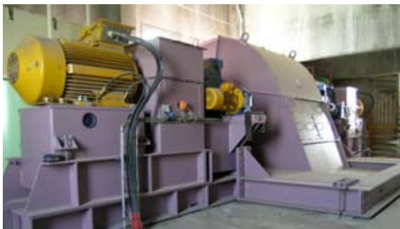
High capacity elevator head (1600 m 3 /h, height 65 m, 2x200 kW)
