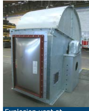
Explosion vent at elevator head
